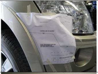
19. To familiarise yourself with the cut line location, do a dry run placing template in position on RHS of vehicle. Note key alignment points to headlamp lower corner, distance to horizontal cut line from lower bumper edge and fender rubber trim edge. Spot mark ends of cut lines to flare and inboard end of cut line to bumper face.
