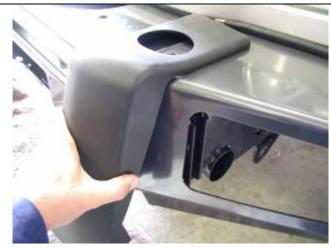
72. Insert the side buffers through the holes and fix using the M6 flange nuts.
