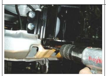
56. Drill Dia 10.0 pinning hole in lower flange of mount bracket into the vehicle crossmember
