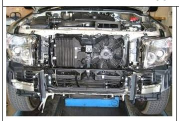
43. Fit mount bracket sets with reinforcing plates to front of vehicle as shown. Use M10 fasteners sets to hold in position.
