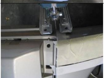
25. Using a jig saw or similar suitable cutting device, cut along the line. The cut through the top of the bumper is aligned with the edge of the buffer recess as shown.
