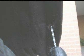
84. Drill holes in fender liner using Dia 7.0 holes in wing return flanges as a guide and fasten fender line with 4 x M6 black bolts, washers and flange nuts.
