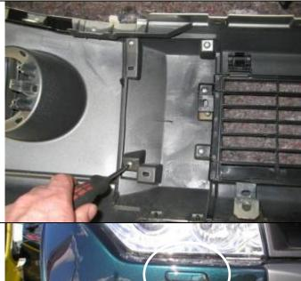
16. Remove the two buffer blocks from the bumper. Fixing screws are accessed from rear of bumper as shown.
