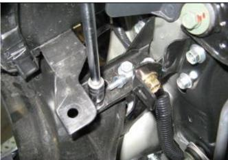
13. Undo upper cross member fasteners as shown on both ends as shown.
