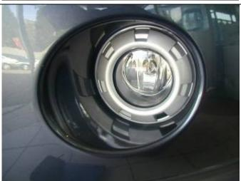
15. If fitted, remove fog lamps including trim rings and set aside.
