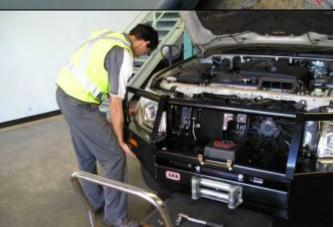
77. Support bull bar on lift device if available or with the help of one or more assistants lift the bull bar into position on the mount brackets.
