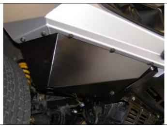
95. Fit the M6 cage nuts to the under wing pans and fit to the underneath of each wing using M6 x 16 Hex bolts, M6 Washers and M6 Spring Washers.
