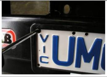
74. Fit number plate using black dome head screws inserted into grommets.
