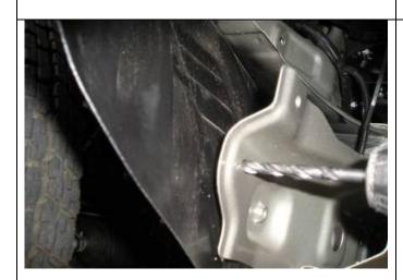
85. Drill hole in fender liner and cross beam as shown and secure liner with M6 black bolts, washers and flange nuts.
