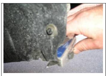
86. Carefully, using a sharp knife or hacksaw trim off the fender liner co-incidental with the lower edge of the cross beam.
