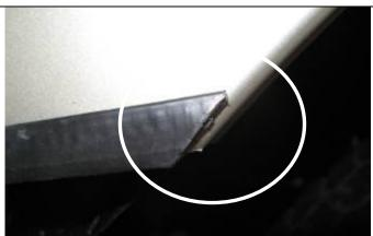
41. Mark and then trim one end of each of the pinch welds to suit the angle of the wheel arch area of the flare. Use a cutting wheel in a grinder as there is a metal spring channel frame inside the pinch weld.
