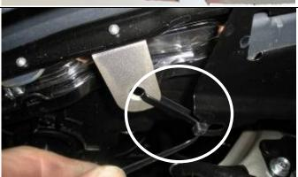
40. To secure inboard end of bumper section, fit a cable tie to the remaining lug on the bumper and through the newly drilled hole in the cross member ends. This cable tie when pulled tighter can adjust the position of the bumper to the bull bar, so wait until after the bar is fitted before trimming the cable tie off.
