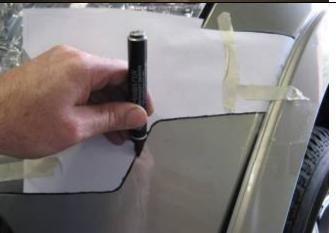
21. Refit template to vehicle and mark cut line (LHS shown).
