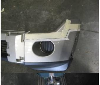
24. Remove bumper and apply masking tape to either side of cut line to prevent damage to bumper when cutting.
