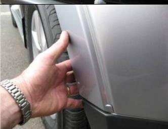
10. Free the end of the flare from the bumper by pulling outward in the lower region as shown.
