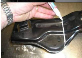
28. Mark cut lines on each end of the cross member. The edge of the cut is 25mm inboard of the M6 hole as shown.
