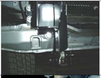
57. Fit M10 SEMS bolt and load flange nut from inside cross member then do up tight.
