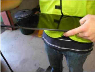
75. Apply rubber mold to edge of winch hole cover panel and trim off excess.
