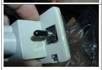
92. Remove indicators from cartons and then remove screws and speed nuts from each light. These fasteners are not to be reused – new screws are supplied in the fitting kit
