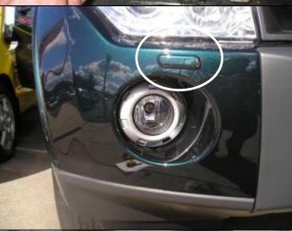
17. If washer assemblies fitted (circled for reference in picture), remove and set aside.
