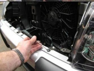
7. Remove upper bumper retaining scrivets.
