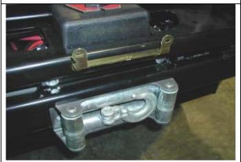
70. Fit number plate bracket as shown using M6 hardware.
