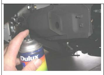
87. Using a black spray pack, paint the exposed color coded area of the cross beam so it does not show.
