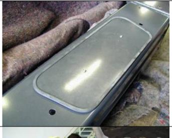
76. Fit panel to top face on bull bar using 2 x M6 dome head stainless steel screws, flange nuts and flat washers.
