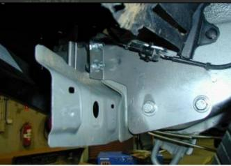
58. Reclip electrical loom connector into new bracket flange both sides of vehicle.
