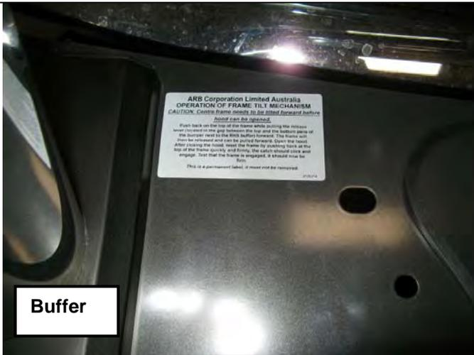
75. Apply the frame tilt operation label to the top face of the pan adjacent to the buffer as shown in diagram
