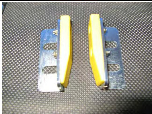
53. Fit a urethane buffer pad to each of the right angle brackets using M4x16 csk head screws and M4 nyloc nuts, to create a pair of RH and LH assemblies as shown.
