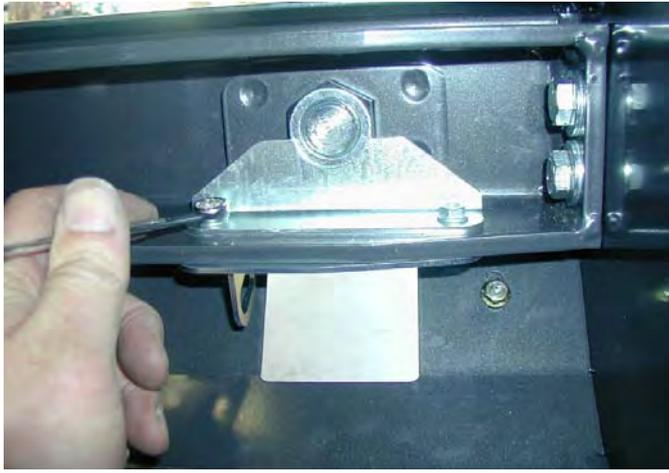
23. When the large nut is in its final position, fit the retaining bracket and secure with the using M6 bolt, washer and flange nut sets.
