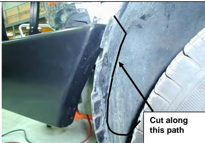
72. Trim fender liner with air hacksaw or similar tool along line as shown so it will pull back inside the wing tip.
