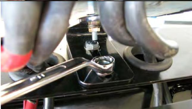
27. Using M8 fasteners fit control box mounting bracket to pan
