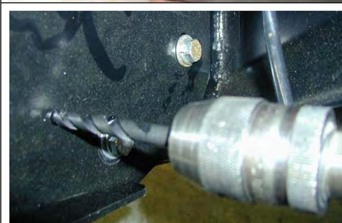
68. Using the M10 pilot holes in mount brackets, drill pinning hole through uprights on bull bar. Fit M10 screw, washer set and flange nut and do up tight.
