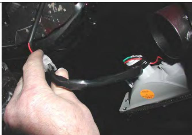
69. Wire up indicators and running lamps. Wire loom extensions are supplied in fitting kit.
