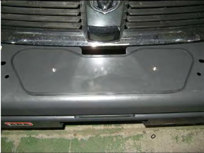
38. Place washers over the winch cover fixing holes located on the top middle face of the winch bumper.
