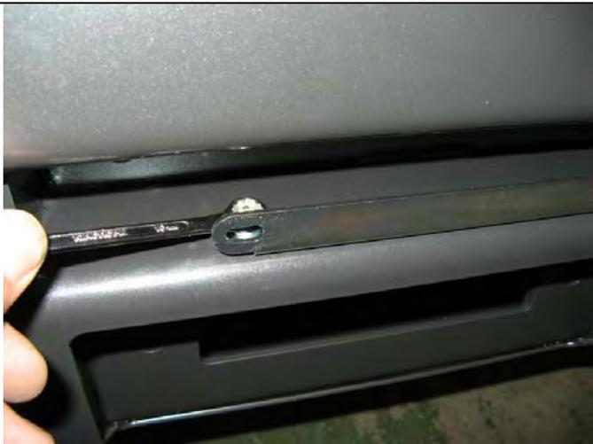
24. Secure the number plate bracket using M6 bolts, flat washers and flange nuts. Attach the longer side to the bullbar and the shorter side to the number plate.
