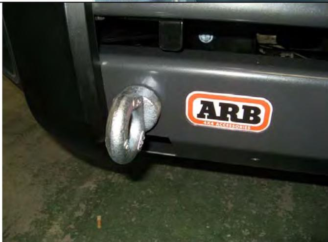
21. Fit large eyebolt nut into the location plate of channel gusset.
