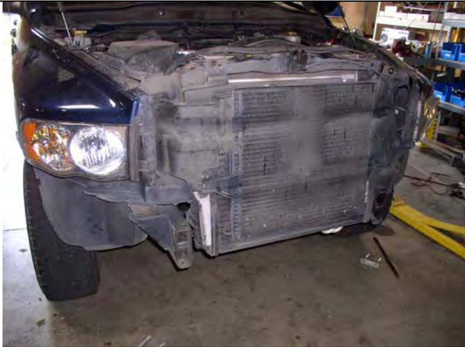
1. If fog lights fitted in bumper, undo fog light loom connection (connection located on LHS of bumper)
