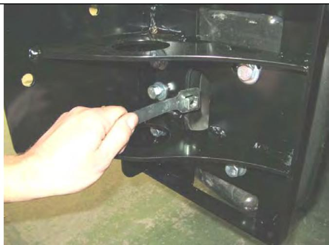
9. For pinning bolt from outboard of reinforcing bracket, fit cage nut plate assembly through into chassis end aperture as shown, then fasten in place through drilled pinning hole with M10 x 30 SEMS bolt and washer set. Do up to specified torque. Repeat for other side of vehicle.
