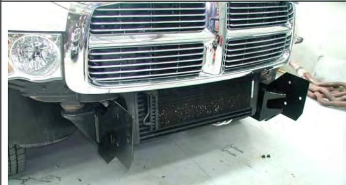
11. Insert original U bolts, entering from **inboard** face of chassis (you may have to tilt intercooler to gain sufficient clearance to allow U bolt to enter this side).
