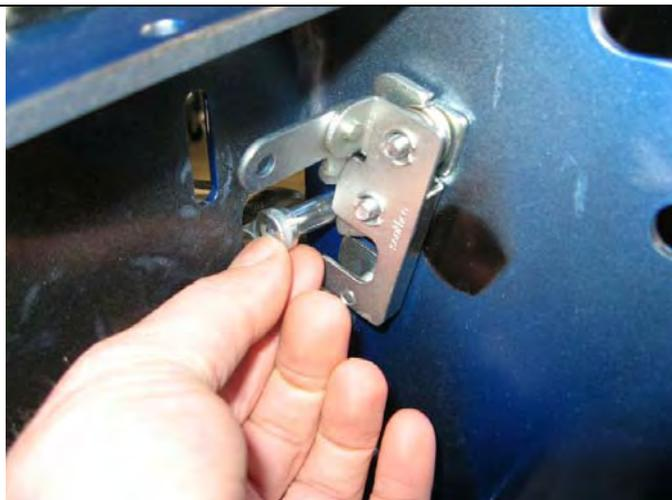
52. Fit the striker pin to the **RHS** hinge plate and secure with 5/16"UNC nut and spring washer as shown and tighten to 22Nm or 16lbft
