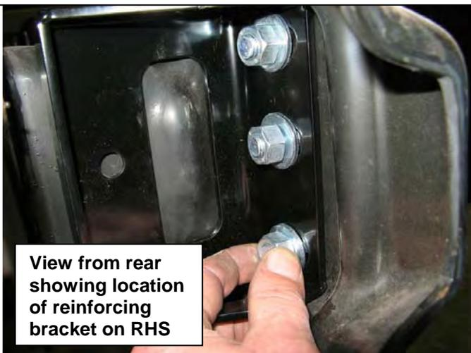
5. Do fasteners up to specified torque, ensuring that reinforcing bracket is sitting snugly against chassis side face.
