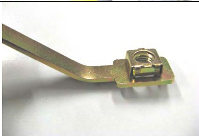
8. Fit the M10 cage nut to nut plate as shown.
