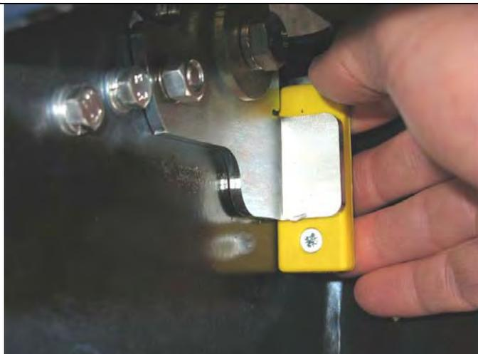
55. Fit the RHS buffer pad assembly as shown, wedge of pad up. Secure with 2 x M8 bolts, washers and flange nut sets. Load bolts from inboard side of upright, nuts are on bracket side.
