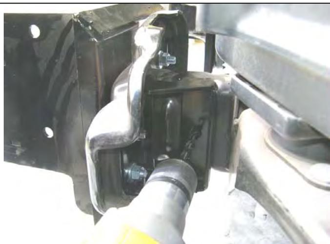
7. Drill 1 x M10 pinning hole in chassis using existing hole in reinforcing bracket as a guide.
