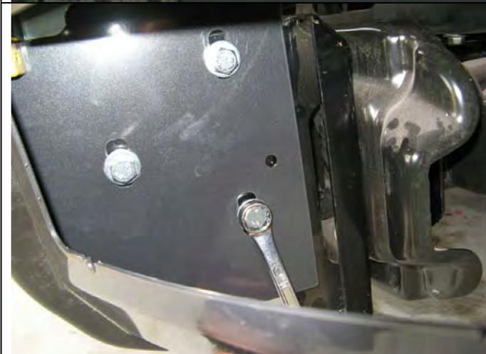
67. When bar is aligned, tighten bolts to specified torque.
