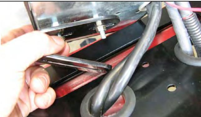
25. Fit large grommets to holes in top pan
