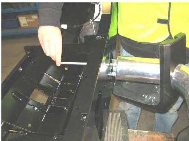
46. Fix the frame to the hinge brackets using 4 x sets M10 x 30 Cap Screws, flat and spring washers
