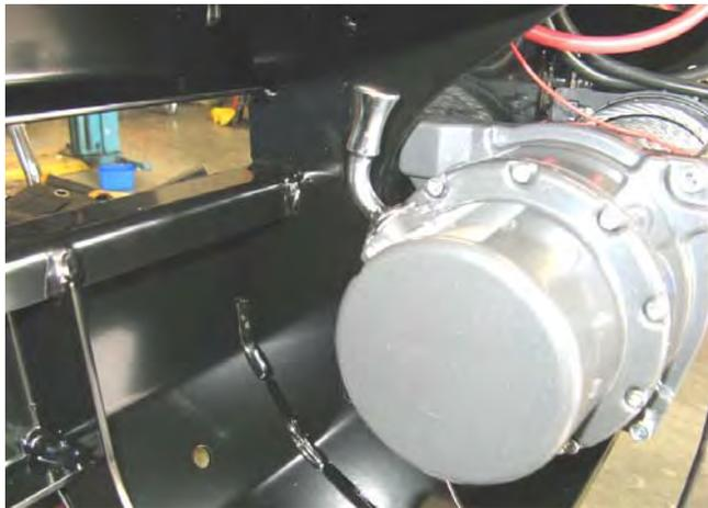
32. Position the winch with the mount face facing upward on an adjustable table or similar and with the assistance of another person lower the bulbar over the winch. The winch handle should be in the LHS of the bull bar for smaller winches than 12-15000lb winches which are on the opposite side as they spool in the opposite direction. The cable must always spool off the bottom of the winch.
