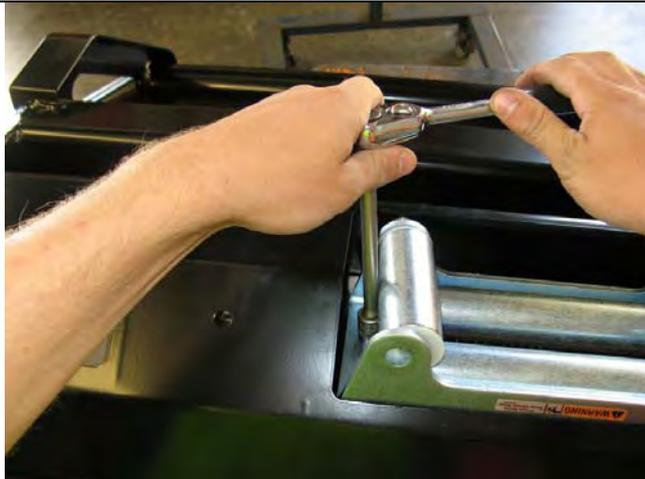
33. Fit the roller fair lead, pull only the end of the cable through and adjust the position of winch then bolt up to specified torque. For 9500 winch, use the 3/8"UNC x 1 1/2" long bolts in the top and supplied 1 3/4" in the lower set through the RFL.
