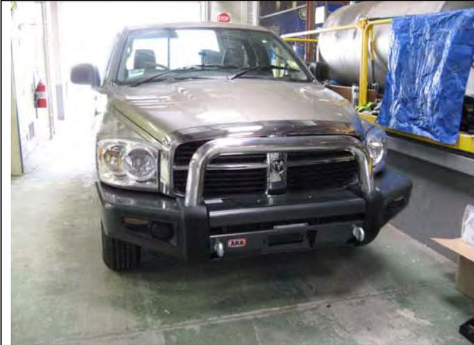
65. Using two people, three if winch fitted, position the bar assembly on the vehicle mounts.
