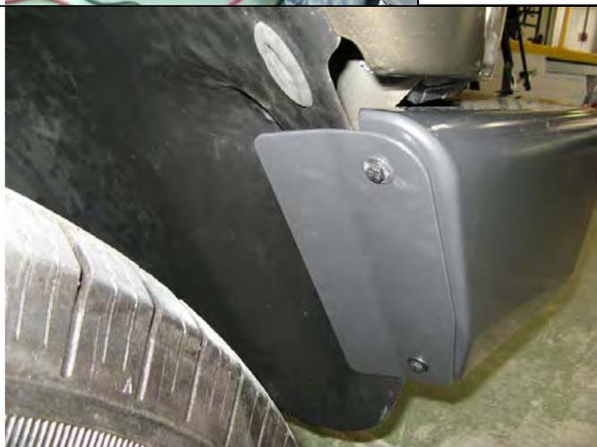
74. Fit liner retainer bracket with black M6 bolt and washer sets into M6 cage nuts in wing returns each side as shown.
