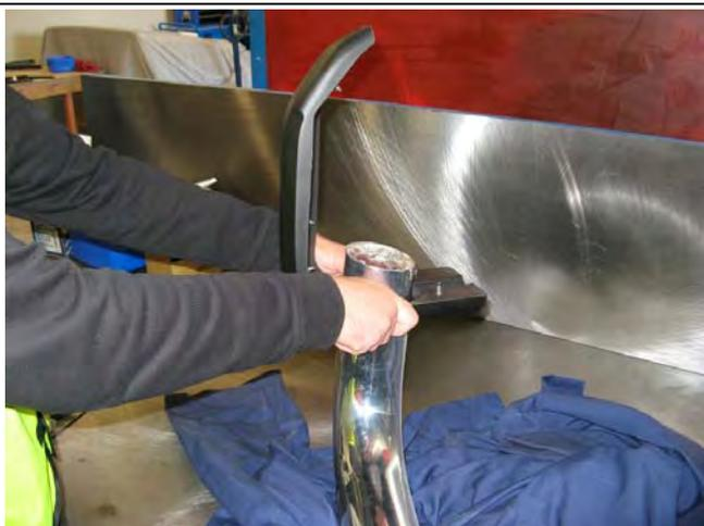
**NOTE:** When the frame sits on the bumper, it is angled backward. Put it up against the bumper and determine which side is LH and RH. The buffers are handed RH and LH. Select the correctly handed buffer to fit over each end of the frame before proceeding.
