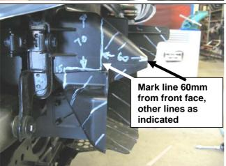
37. Mark the lower section of the air scoop for the power steering radiator as shown. This is for trimming to clear the mount brackets.
