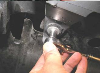
6. Remove lower bumper retaining screws.
