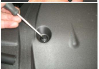
7. Remove plastic engine bay cover above grille area and set aside. Prise open plastic plugs with small flat blade screwdriver or similar as shown.
