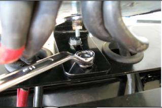
50. Using M8 fasteners fit control box mounting bracket to pan
