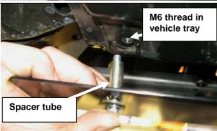
94. Fit stone tray using 4 x M6 bolts and washer sets at front under bull bar and 2 x M6 x 40 bolts, washers and 18mm long tube spacers at two locations into existing sump guard front section as shown.
