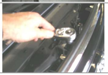
8. Remove 3 X retaining screws from top of grille
