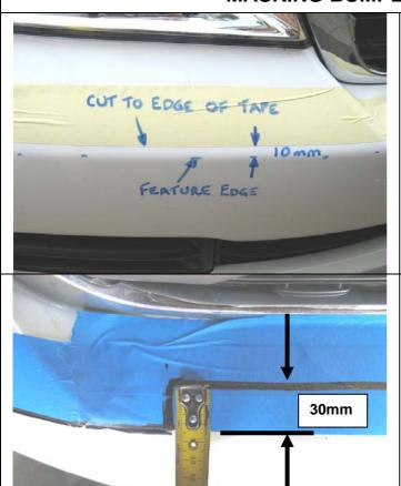
Apply wide masking tape edge, carefully aligning 10mm above bumper feature line as shown. Keep the same line level through the centre section of the bumper as shown
