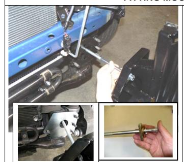
Hint: Check that the M12 long bolts screw freely into the clevis nut threads before assembly.
