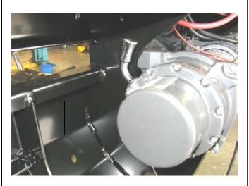
55. Position the winch with the mount face facing upward on an adjustable table or similar and with the assistance of another person lower the bulbar over the winch. The winch handle should be in the LHS of the bull bar for all winches except 12000lb winch is on the opposite side. The cable must spool off the bottom of the winch.
