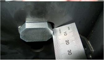
70. The nut when positioned has a slot which should snugly fit and locate the nut on the *outboard* edge of the rectangular chassis hole. The nut should protrude approximately 7mm. Screw the clevis bolt into the clevis nut, *do not tighten yet.*
