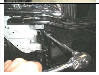
38. Remove scoop and cut using jigsaw or similar and remove burrs.
