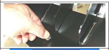
60. Fit 4 x M6 cage nuts to bottom inside face of lower pan in square holes as shown.
