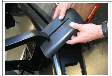
64. Carefully slide top section of buffer past edge of cover strap as shown
