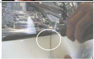
21. Push bumper down immediately below headlamp to gain access with a small flat blade screwdriver and release holding tab.
