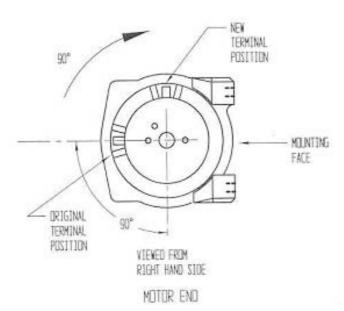
13 The winch motor must also be rotated 90 degrees in a clockwise direction when viewed from the motor end.
