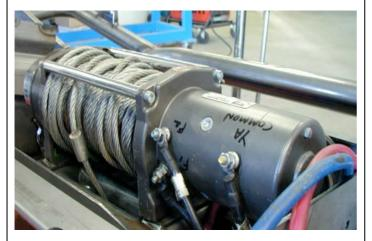
14 With the roller fair lead previously in position, lift the winch into position and bolt into place using the 3/8" hardware supplied with the winch, bolt securely in place.
