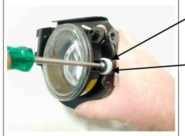
Fit the "u" nuts to the fog lamp bracket , the nylon washer fits between the bracket and the lamp mounting foot ( located on the adjustment side ) fit the fog lamp with the screws provided . Fit the screw covers over the exposed end of the screws in 3 places to each bracket.
