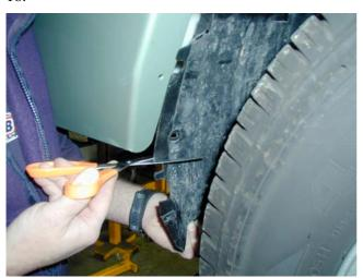
18 Trim the plastic inner guard liners by aligning with the bull bar and using the hole in the wing as a guide, drill a 6 mm hole and secure with the M6 hardware supplied.
