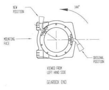
12 To place the winch clutch handle in an accessible location, the gearbox must be rotated 2 bolt spaces (144 degrees) in an anti-clockwise direction when viewed from the gear box end.
