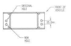
11 **WINCH BAR ONLY** The roller fair lead must be drilled prior to fitment, it can then be assembled into the front of the bull bar along with the winch as detailed in step 14.
