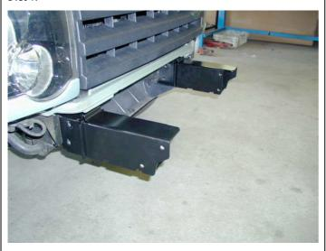
3. Fit the new impact absorbers to both the LH & RH chassis rails . **Note the profiled edge faces outward** Using the 7/16 hardware supplied , bolt the RH impact absorber into position .
