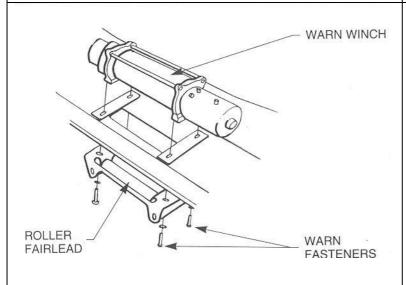
Install the winch and roller fairlead using, bolts, nuts and spring washers supplied by Warn, and 3/8" flat washers (4 off) supplied in bolt kit. Refer to Warn installation instructions for correct procedure. Adjust winch in slots until winch clutch lever can rotate freely in air vent opening on bull bar.
