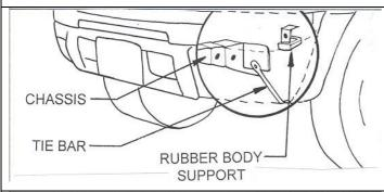
Remove existing bumper from vehicle by removing chassis bolts, outer tie bars and bolts connecting rubber body supports to the vehicle.
