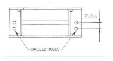
The roller fairlead must have new holes drilled to allow for correct wire rope angle. Using a 12mm diameter drill bit, redrill the fairlead in the position shown in the diagram.
