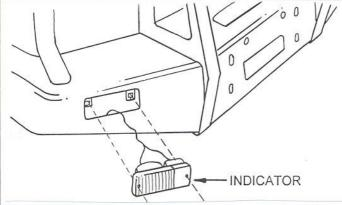
Fit plastic screw plugs provided in indicator kit to bull bar and install indicator lamps using self tapping screws provided with lamps.
