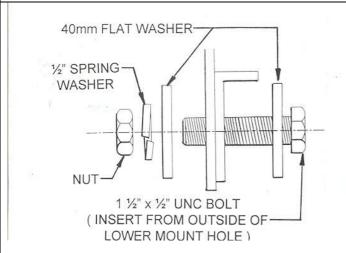
Bolt through lower mount hole using the 1 ½" x ½" UNC bolts, spring washer, nut (2 of each item) and 13 x 40mm flat washer (4 off). Bolt through hole from outside as per diagram, diagram has passenger side drawn.
