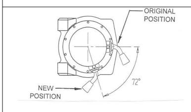
To place winch clutch handle in a convenient location the winch gearbox must be rotated 2 hole spacings, 72 degrees, in a <u>clockwise</u> direction. Place winch on its end and remove all gearbox bolts. Gently raise gearbox just enough to rotate it. Do not completely remove gearbox and avoid damage to the gasket. Refit all bolts and tighten
