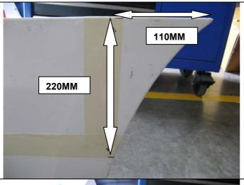
5. From the top front edge of the bumper measure towards the rear 110mm and make a mark. From this point measure down 220mm and mark. This is the cut line.
