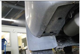
Remove vehicle bumper, mud flaps, tie down hooks and bumper brackets. Retain both mudflaps as they will be needed later. If your vehicle has the Pintle hook remove this also.
