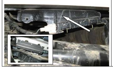
Remove this bracket from vehicle (shown with arrow) and relocate with new bracket supplied in kit. Make sure all wires are clear of the exhaust. Relocation bracket fitted to vehicle shown inset.
