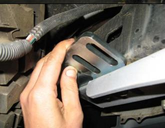
16. Place the 8mm packers between bar mount and chassis then tighten.
