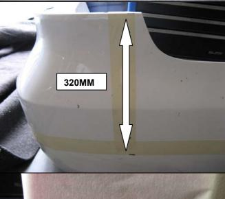
6. From the top edge of the bar measure straight down 320mm and mark. Join marked lines with a length of masking tape making sure it is straight. This will be the cut line.
