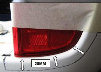
7. From the edge of the fog light/reflector measure and mark several points 20mm away from the lens. Join these marks to form a line as shown in the photo.
