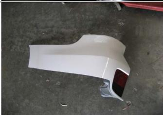
10. Using an air operated hacksaw or small grinder with a cutting wheel cut the bumper using the marked lines.
