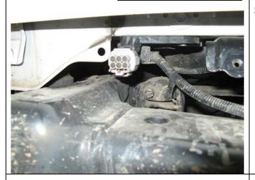
3. Locate the six pin plug on the left hand side and un-clip from its mount. Using a zip tie attach it to the loom that runs next to it. This is to clear the front face of the rear bar.
