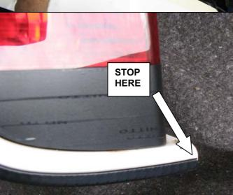
12. Apply pinch weld to cut surface stopping at the base of the fog light as shown. Fit bumper back on vehicle.
