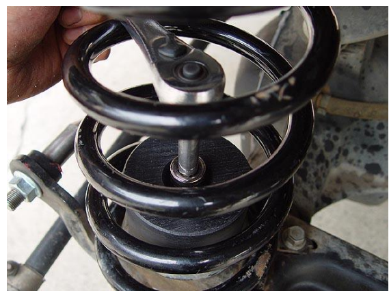
Img.8 front lower bumpstop extension
