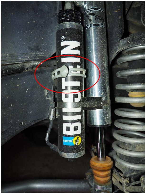
Img.1: front reservoir holder and crooked reservoir
