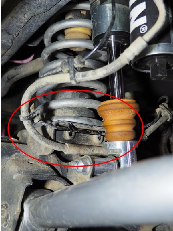
Img.4: front brakeline and abs line bracket at axle
