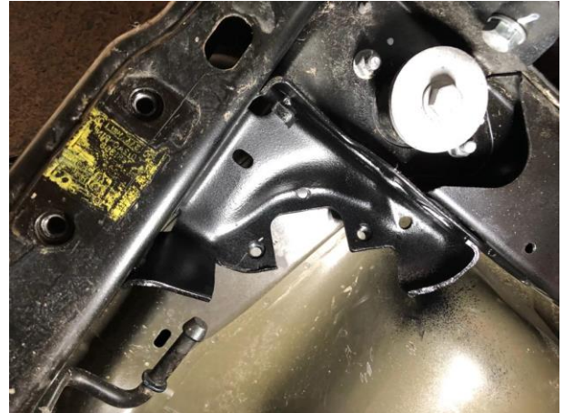
Img.6: JK rear upper shock relocater – cuts
