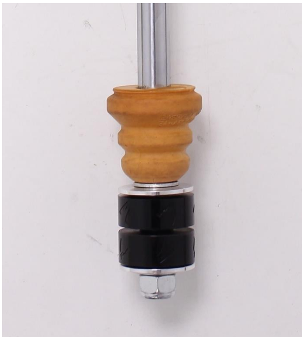
Img.2: bushings on pin at rod
