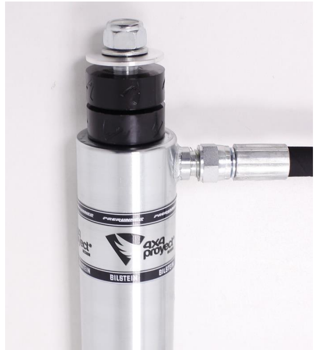
Img.3: bushings on pin at body
