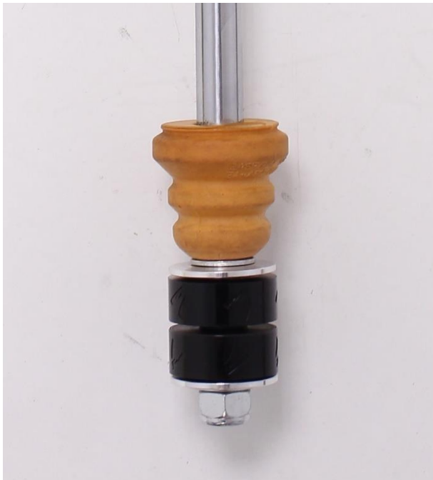
Img.2: bushings on pin at rod
