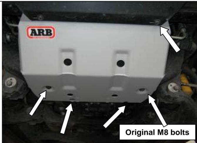
5. Mount front panel to vehicle using original bolts and positions. If fitted with an ARB bar place panel on top side of bullbar stone shield. Leave bolts finger tight.
