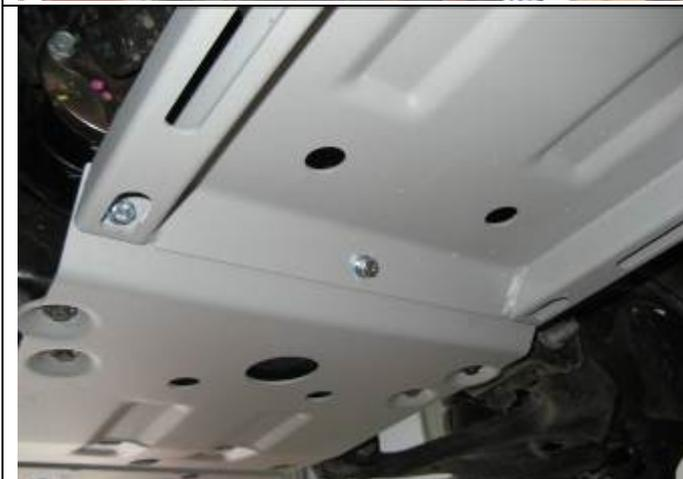
10. Lift transmission panel into place and secure to sump panel using 3 x M8 bolts, spring washers and flat washers supplied. Leave finger tight.
