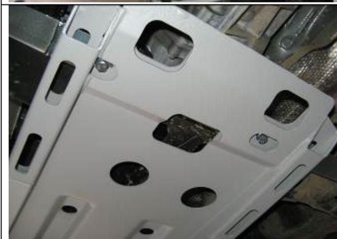
11. Secure panel to mounting bracket using 2 x M8 bolts, spring washers, flat washers AND flange nuts supplied. **When satisfied tighten all bolts to specified torque.**
