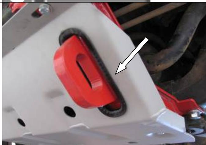
3. Fit rubber edging as shown before fitting panel to vehicle.
