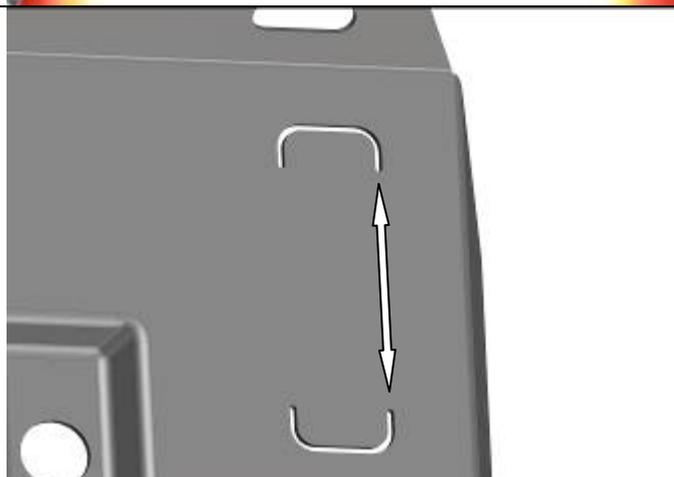
2. Using a marker pen and ruler joint the two 'U' shaped cut outs. Use masking tape to cover the outside edges of the drawn lines. Cut along lines using grinder with cutting disc to remove the rectangular section. De-burr and paint edges.
