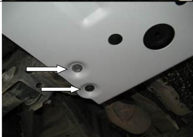
6. Fitting sump panel. As per step 2 fit an M8 cage nut to centre rear of panel. Lift panel into position and secure to cross member using original M8 bolts as shown. Leave finger tight.
