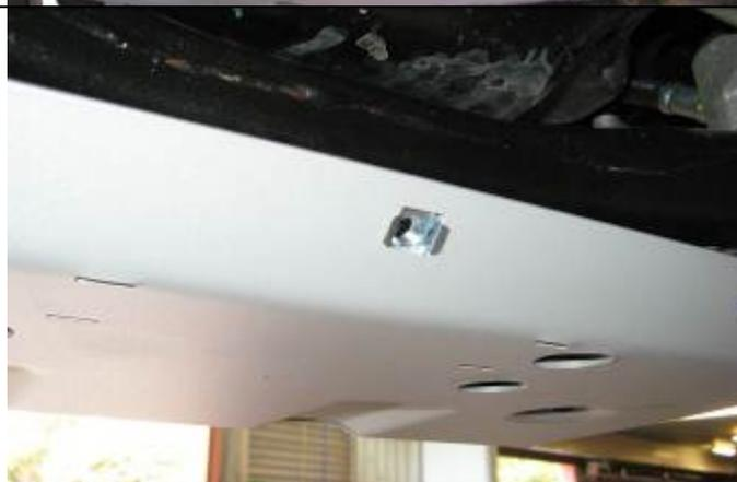
4. Fit M8 cage nut to centre point on rear of panel.
