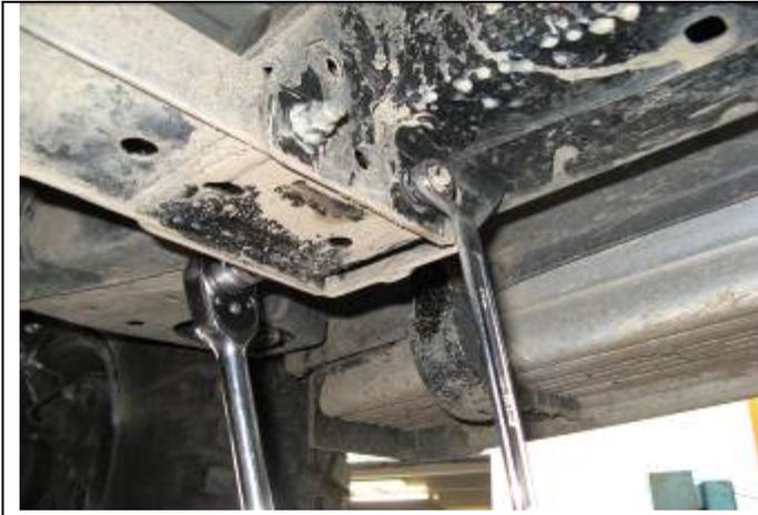
8. Before fitting transmission panel the mounting bracket needs to be attached to the rear of cross member. As shown in photo remove mounting nuts from gearbox cross member. **NOTE:** If you have side rails fitted it may be required to orientate bolts so they are placed in from front to back.
