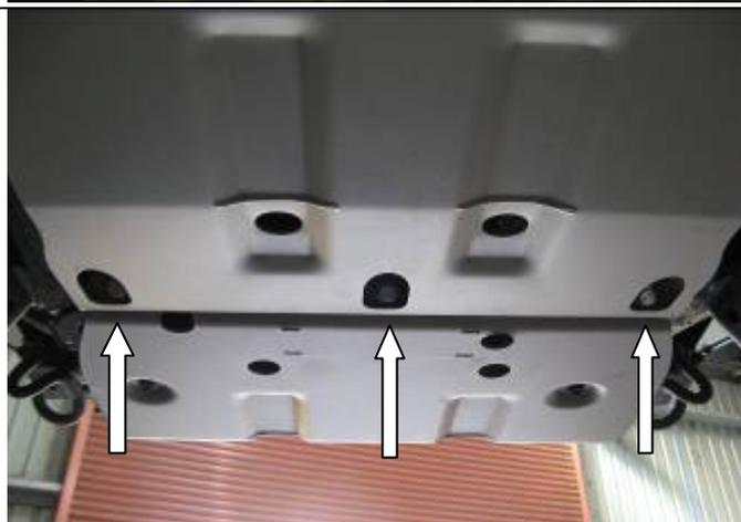
7. Secure front of sump panel to front panel using 3 x M8 bolts, spring washers and flat washer supplied, **tighten to specified torque**. Use M8 flange nuts on outer holes.
