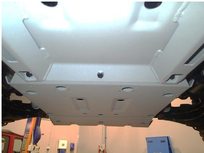
Connect transmission panel
