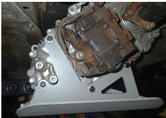
Transfer case panel rear side
