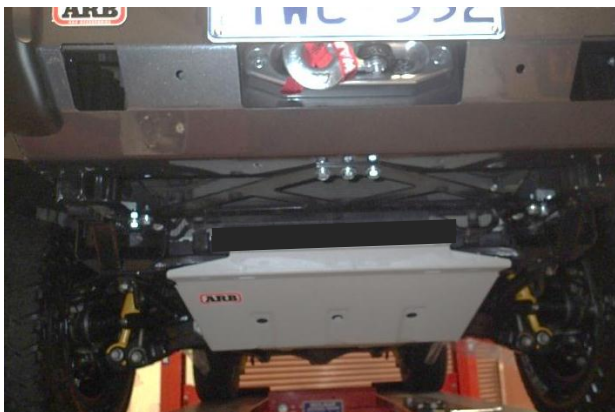
Fit front panel to vehicle
