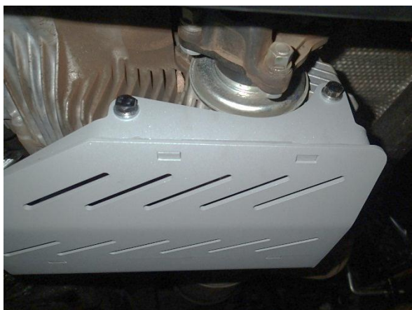
Transfer case panel front side
