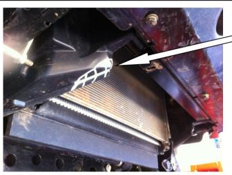
Trim plastic air dam using an air saw / knife.
