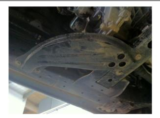
Remove and discard OEM shield from 16. transfer case.
