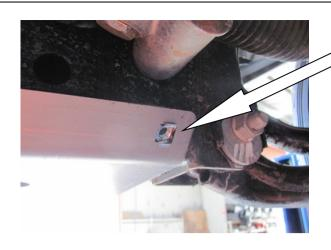
Remove original stone shields from vehicle. Insert  $3 \times \emptyset$  M8 cage nuts to rear of supplied front panel as shown.
