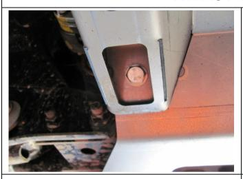
13. With the help of another person or a jack lift the transmission panel into place and secure the front section using 3 x Ø M8 x 25 bolts, spring washer, flat washers and flange nuts.
