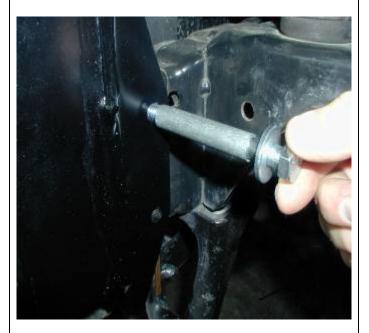
31. Insert the bolt & washer and crush tube into the side pinning hole and align it with hole on the inboard side and push it thru the entire width of the chassis.
