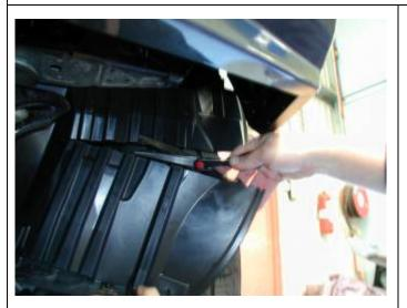
62. With part of the inner guard now trimmed to clear the wing return the remaining part of the inner liner that hangs down below the bottom of the wing can be trimmed off horizontally.
