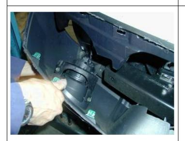
7. With the first cut completed on the outer bumper cover, the fog lamp loom (where fog lamps are fitted) can be accessed & dis-connected both sides. The lower bumper bar is now free and can be removed .Using a No 20 TORX bit remove the fog lamps from the lower bumper section.
