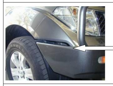
45. Ensure the bull is sitting on the vehicle level and the gap between the bumper bar and the bull bar wing is parallel.
