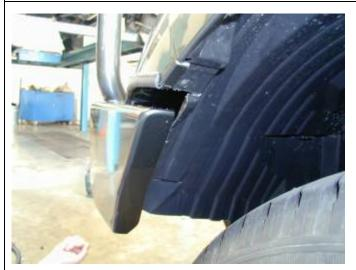
63. Push the outer edge of the liner forward past the wing return edge so that it snaps in against the wing brace as shown.
