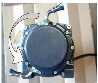
32. Remove the cap head screws retaining the gearbox to the winch drum. Carefully lift the gearbox a small amount (5 mm) and rotate144 degrees counter clockwise (four hole spacings) and re-fit the cap screws. This places the winch handle in the correct orientation.
