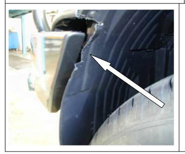
61. With the two horizontal cuts complete, cut down from the end of the top cut to the bottom cut vertically (the inner guard needs to have clearance to the bull bar wing return as shown).
