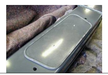
36. Fit panel to top face on bull bar using 2 x M6 dome head stainless steel screws, flange nuts and flat washers.
