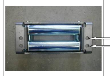
35. Using a 12mm drill bit, mark & drill two new holes in the roller fairlead 25mm below the original holes.
