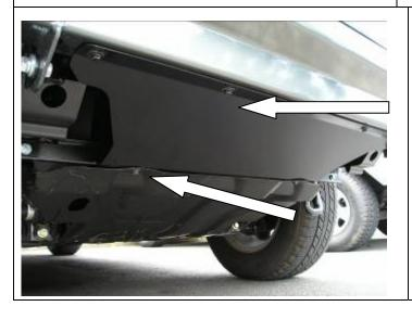
55. Attach the stone tray to the under side of the bull bar with the black M6 bolts, flat washers & spring washers.
