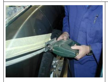
6. Using an electric jig saw with a fine cutting blade - use the top of the 12mm tape as the cutting line. Start the cut in the wheel arch area as shown working from one side to the other. Cut thru both the back edge of the bumper and the plastic guard liner. An assistant at this stage could hold the bumper cover in place to ensure a straight & level cut. Ensure hearing and eye protection is used.
