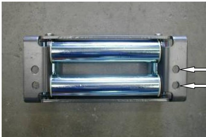
46. Using a 12mm drill bit, mark & drill two new holes in the roller fairlead 25mm below the original holes.
