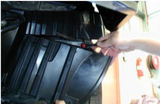
73. With part of the inner guard now trimmed to clear the wing return the remaining part of the inner liner that hangs down below the bottom of the wing can be trimmed off horizontally.
