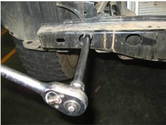
25. The four bolts that hold the bumper reinforcement beam can now be removed and set aside.
