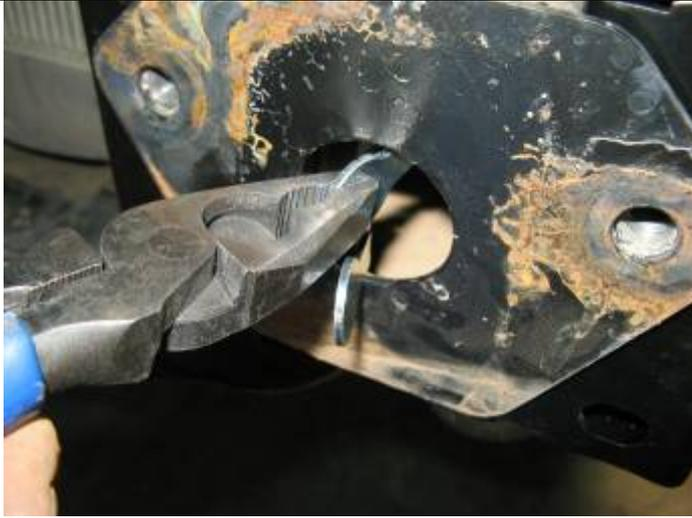
33. Bend back tabs on nut plates back into chassis ends with pliers as shown
