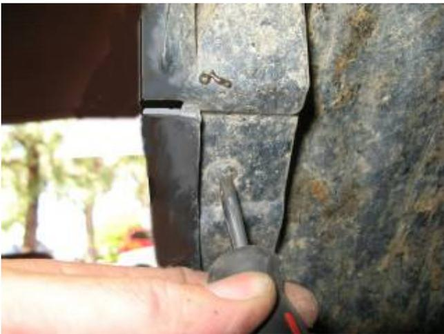
6. Remove the screws securing the fender liners to bumper in the forward wheel arch areas
