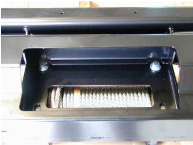
44. Lay the winch on a suitable flat surface and place the bull bar on top so that the wire rope will feed thru from the bottom.
