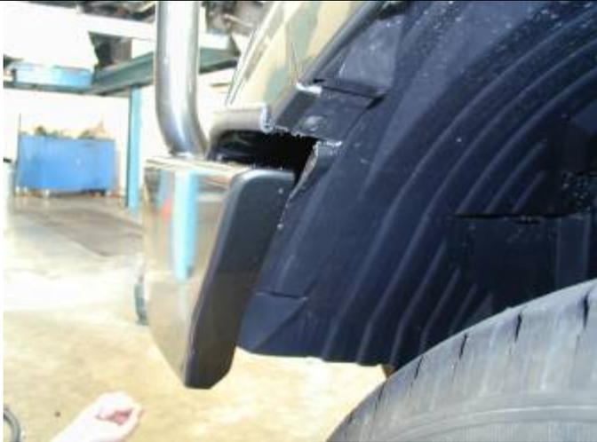
74. Push the outer edge of the liner forward past the wing return edge so that it snaps in against the wing brace as shown.
