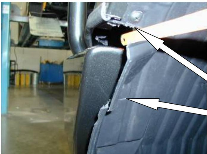
70. Using a hack saw blade or a sharp knife extend the top horizontal cut from the jig saw in towards the centre of the car.
