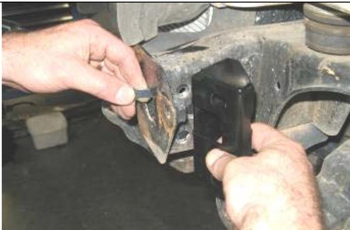
29. Fit one hand of a pair of reinforcing brackets up against the side of chassis and chassis end plate as shown
