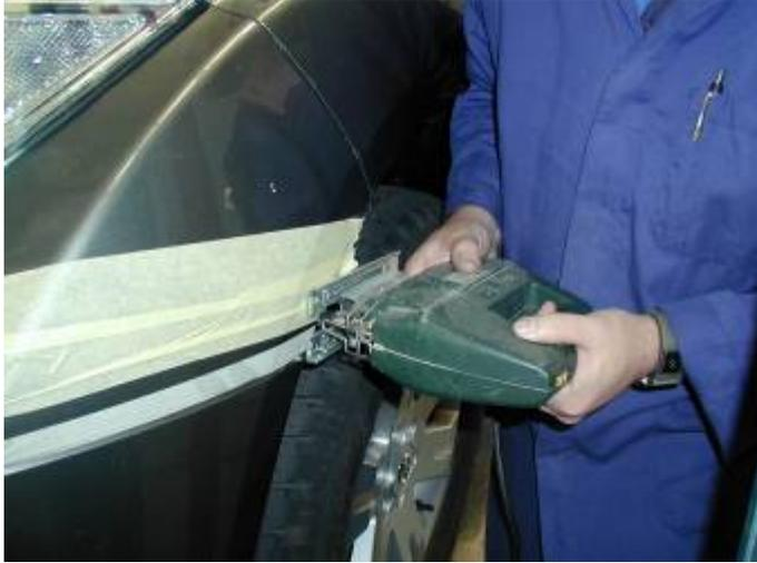
11. Using an electric jig saw with a fine cutting blade - use the top of the 12mm tape as the cutting line. Start the cut in the wheel arch area as shown working from one side to the edge of the centre section to be cut by hand. Cut through both the back edge of the bumper and the plastic guard liner. An assistant at this stage could hold the bumper cover in place to ensure a straight & level cut. Ensure hearing and eye protection is used.
