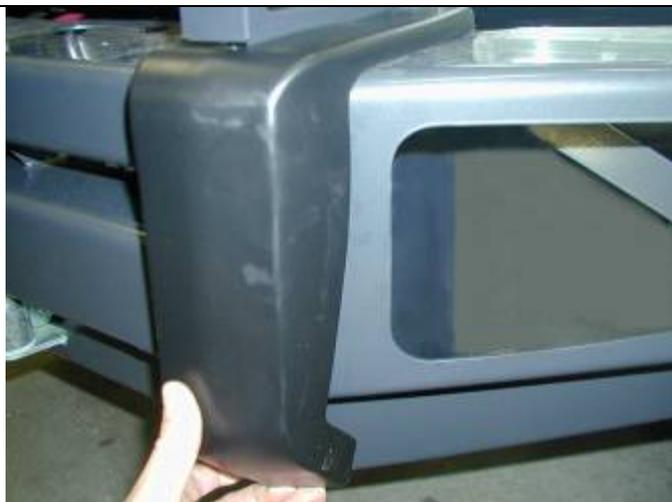
39. Fit the buffers to either side of the bull bar using 6 x M6 flange nuts. Do not over tighten.
