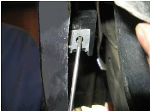
7. Remove the speed nut from the bumper on each side
