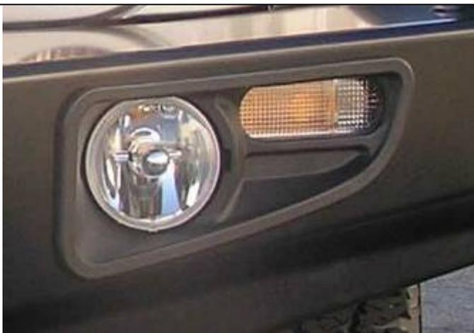
65. Assemble and install combination light surrounds (p/n 3163015) as per instructions no. 3786421 supplied with surround kit. Note: Optional fog lamps can be installed at this point as per fitting instruction no. 3783315 supplied with fog lamp kit no. 6821201.
