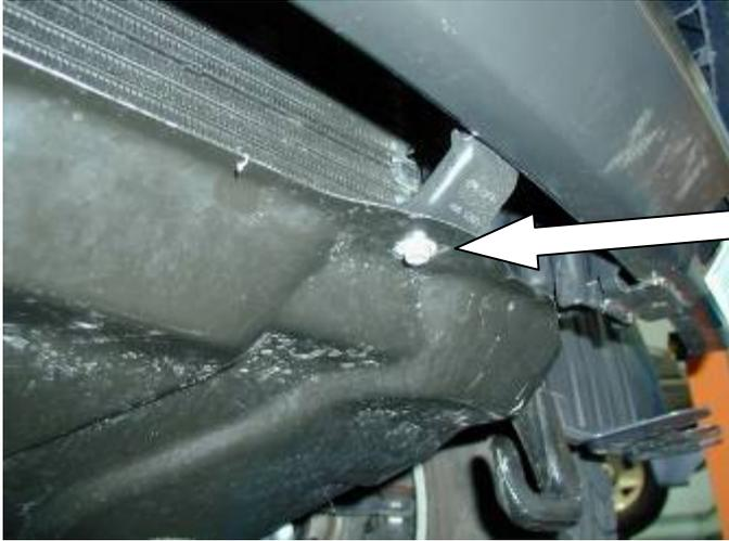
23. The bumper reinforcement beam is now visible. Remove the two bolts that hold the factory steel stone tray to the beam and lower the front edge of the stone tray down passed the recovery hook.
