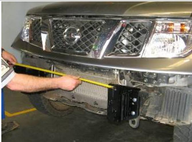
37. Align the brackets ensuring that the packer plates are firmly pushed in and nip up the M10 bolts.
