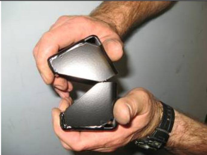
28. Break apart each of the bracket sets as shown. These are handed to fit around the weld nut on the rear of the chassis end plate.
