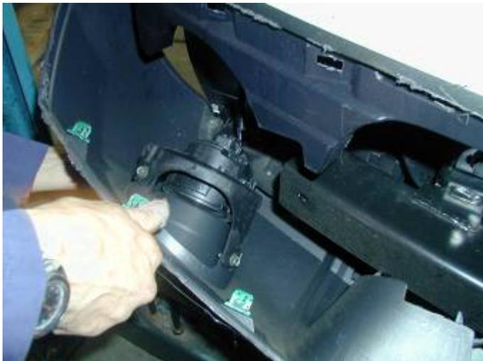
13. With the cuts completed and the bumper supported, disconnect the fog lamp loom
