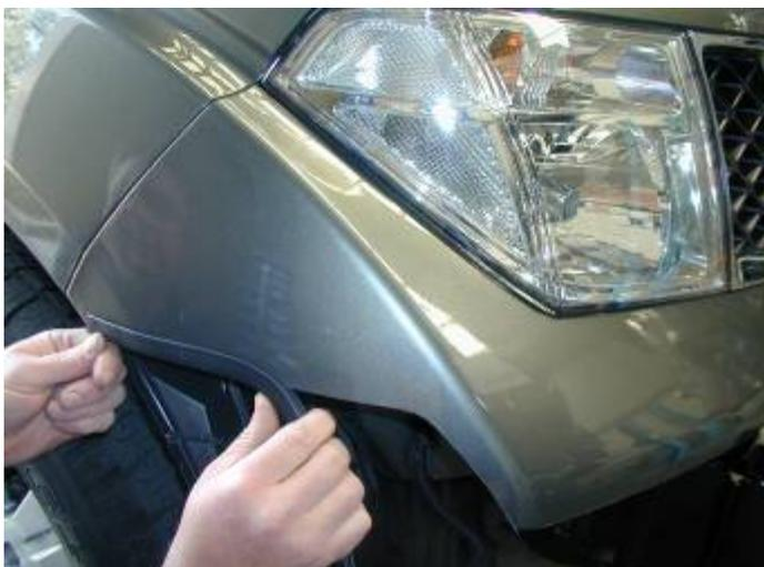
21. The pinch weld trim can now be attached to the cut area.
