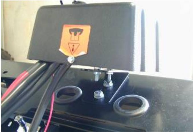
50. Attach the control box to the control box bracket as shown.
