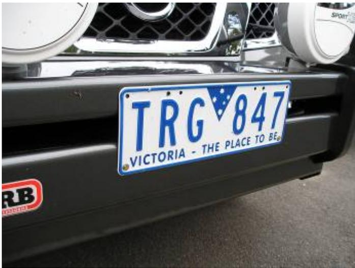
68. The number plate can now be attached to the bull bar. Using the two plastic square plugs supplied, push them into the two square holes in the face of the bull bar. Position the number plate as shown - using the two lower outer holes.
