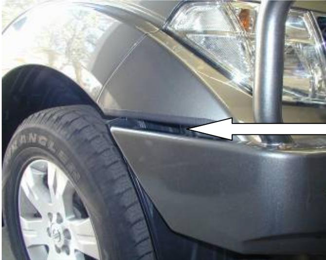
57. Ensure the bull is sitting on the vehicle level and the gap between the bumper bar and the bull bar wing is parallel.
