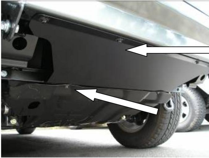
67. Attach the stone tray to the under side of the bull bar with the black M6 bolts, flat washers & spring washers.
