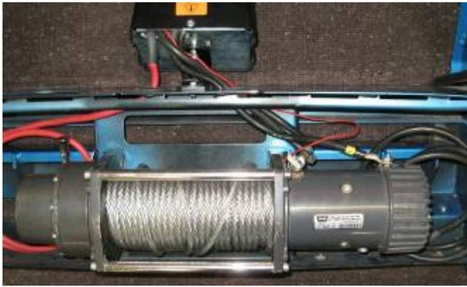
52. Run the cables through the rubber grommets and connect to the winch as per the wiring diagram supplied with the winch.
