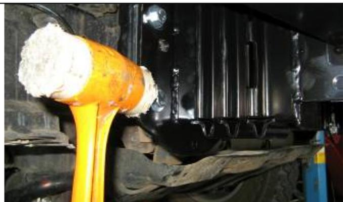
56. If the bull bar is not central to the vehicle, tap the outer corners of the mount bracket flanges as shown.
