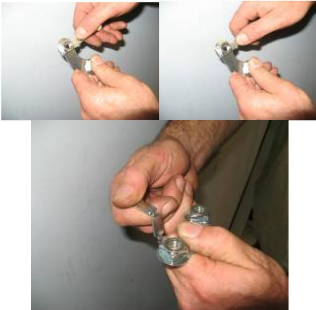
26. Bend up the tabs on each of the four nut plates as shown in two stages.
