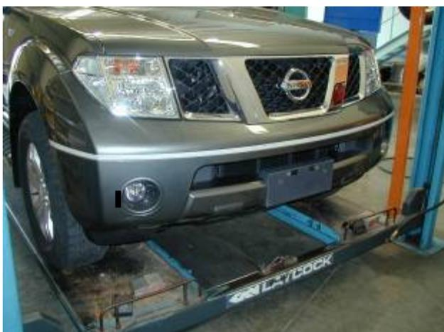
8. Using the bumper bar "grooved highlight line" as a guide run the 12 mm wide masking tape from the fender opening from the left hand side across to the right hand side as shown. Align the lower edge of the tape with the groove in the bumper.
