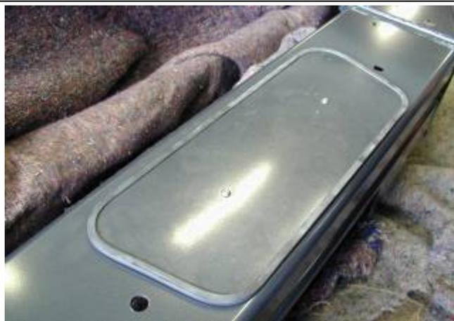
42. Fit panel to top face on bull bar using 2 x M6 dome head stainless steel screws, flange nuts and flat washers.
