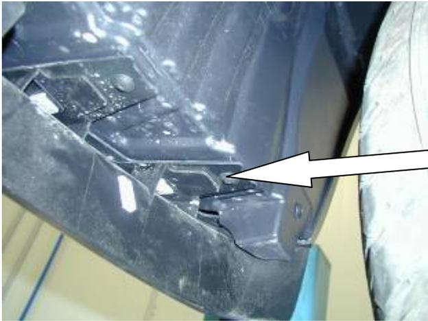
5. Remove the two bolts and screw from the fender opening area each side that attaches the bumper bar to the plastic inner guard liner as shown.
