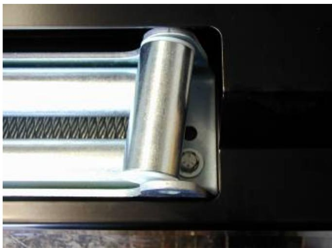
47. Remove the cir clips from the bottom of the vertical rollers of the fairlead and push the pin upwards. Push the vertical rollers inwards on the lower edges as shown and using two 3/8" x 1 3/4" bolts M10 flat and spring washers, attach the lower section of the roller fairlead to the bull bar and winch.
