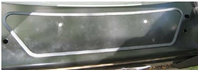
51. Fit panel to top face on bull bar using stainless steel 2 x M6 dome head screws and stainless steel flat washers and flange nuts.
