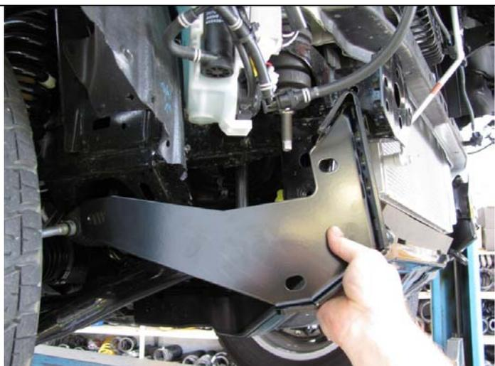
33. Fit handed specific side braces as shown, locating over the captive nuts at the rear of the chassis.
