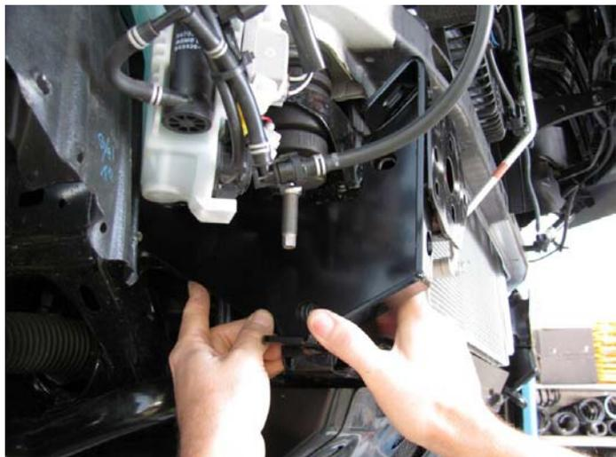
34. When side braces are fitted in position as shown, insert ***fine thread M12 x1.25P x 30 bolt*** and washer sets into lowest hole position to chassis. There is an existing captive nut in chassis, ***but do not do up tight.***
