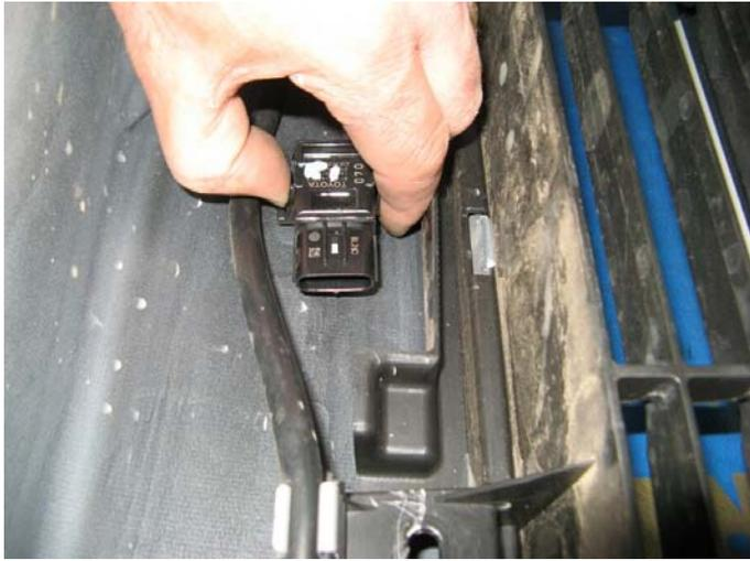
22. **If parking sensors fitted**, mark each sensor for identifying position in bumper, then **carefully** remove sensors, disconnecting from the harness first, then unclipping the sensor from the holding sleeve, finally remove the sleeves from the bumper holes
