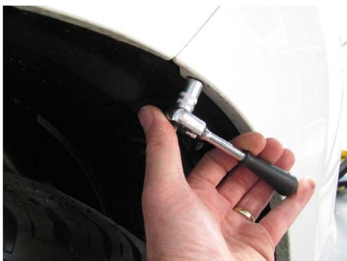
17. Remove the screws securing the bumper to wheel arch area and across the lower section across the front so that there are no more fasteners securing the bumper
