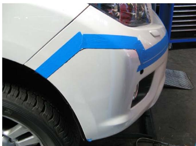
10. Apply 50mm masking tape along the top side of the cutting line right across the bumper as shown
