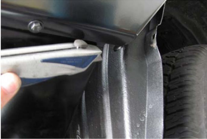
88. Push the outer edge of the liner forward past the wing return edge so that it snaps in place
