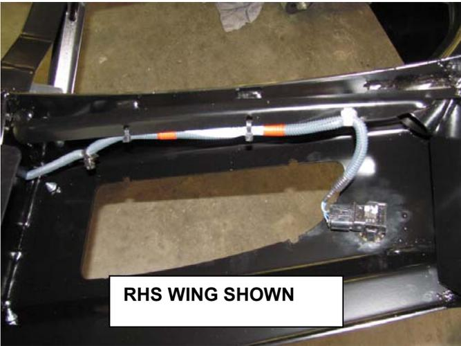
45. Fit the sensor sleeves, then fit sensors into original positions as marked
