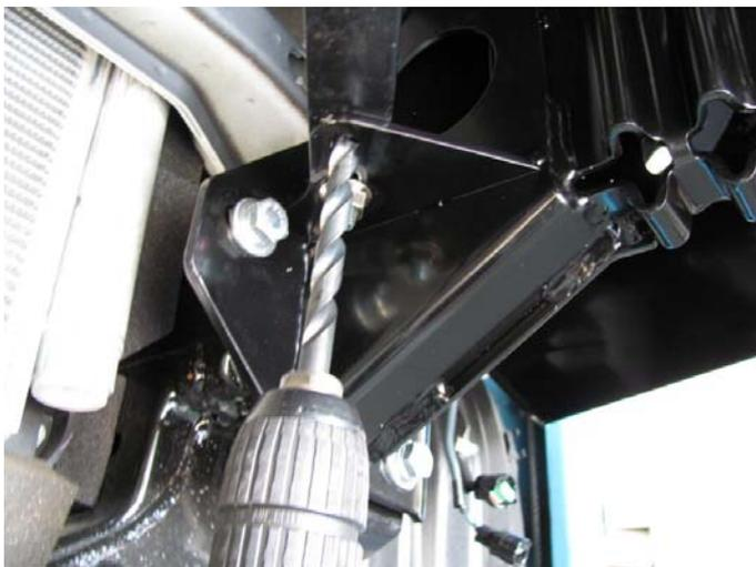
72. Using a Dia10mm drill bit, drill and pin the straps at the adjustment end using the pilot hole as a guide, as shown (note strap fits above the gusset as shown).
