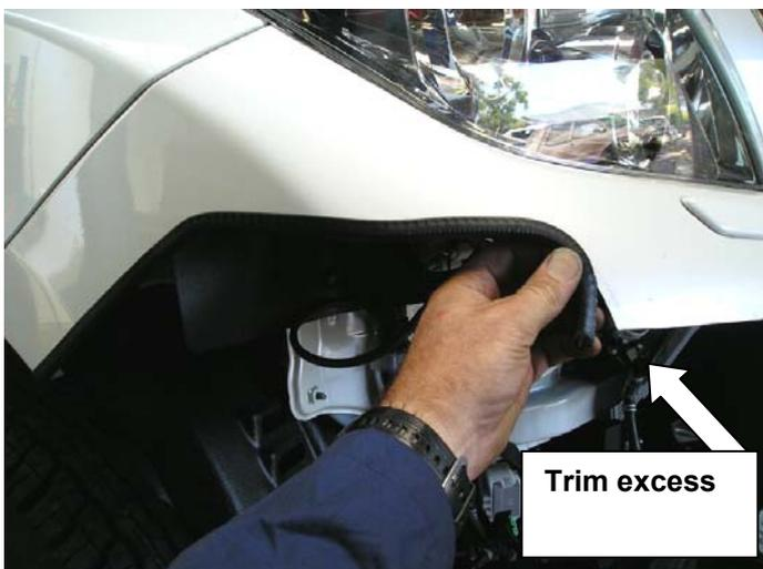
42. Fit pinch weld to cut area as shown, trim to length.
