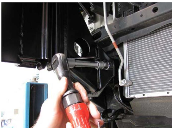
37. Fit impact absorbers to chassis ends using ***fine thread M10 x 1.25P x 30 bolt*** and washer sets supplied, note that the brackets are handed, slide them towards the centre of the vehicle on the adjustment slots ***do not do up tight***
