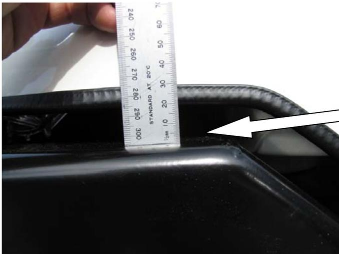
66. Ensure the bull bar is sitting on the vehicle level and the gap between the bumper bar cut and the bull bar wing is even.
