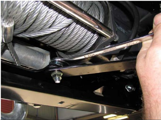
71. Fit the two bracing straps from the top face of the gusset on the mounting bracket to the bottom of the flange on the rear of the winch bracket in bull bar
