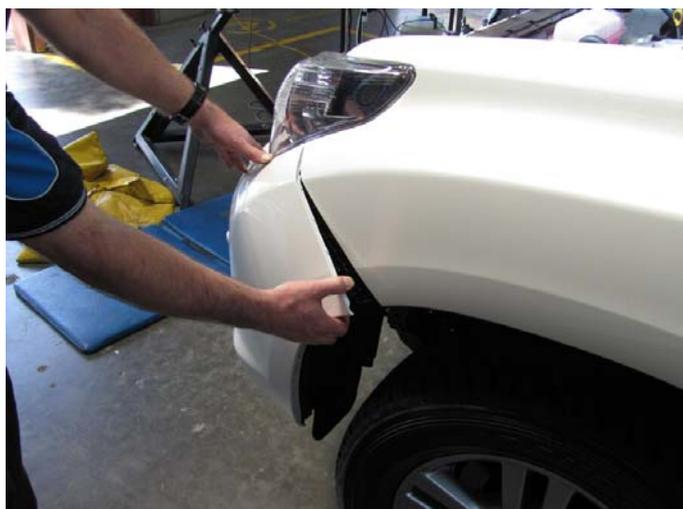
20. Carefully, and ideally with the aid of a friend, unclip each outer of the bumper at the guard as shown and remove bumper.
