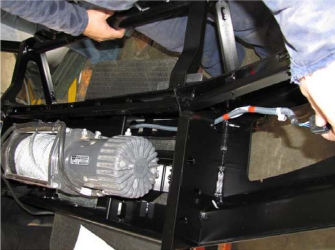
43. Route the sensor loom through the Dia 38mm holes in the bull bar provided in the uprights top forward position, and the top holes in the side of the winch bracket.
