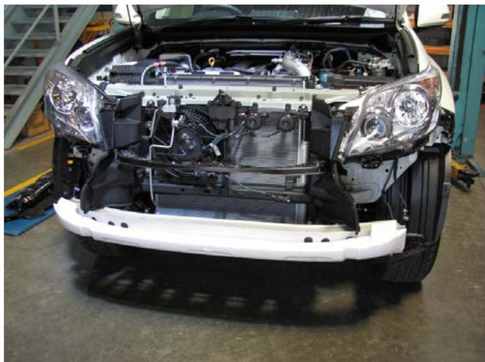
26. Remove reinforcing beam foam pad, then remove the beam, *refer next step.*
