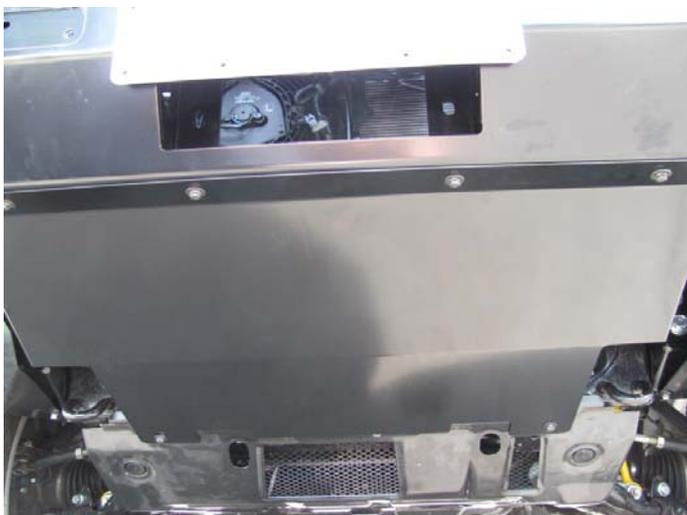
82. The stone shield can now be fitted using 6 x M6 bolt and washer sets
