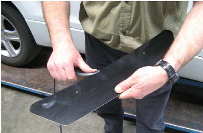
50. Apply rubber mould to edge of winch hole cover panel and trim off excess.
