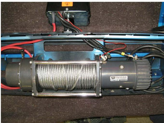
61. Run the cables through the rubber grommets and connect to the winch as per the wiring diagram supplied with the winch.
