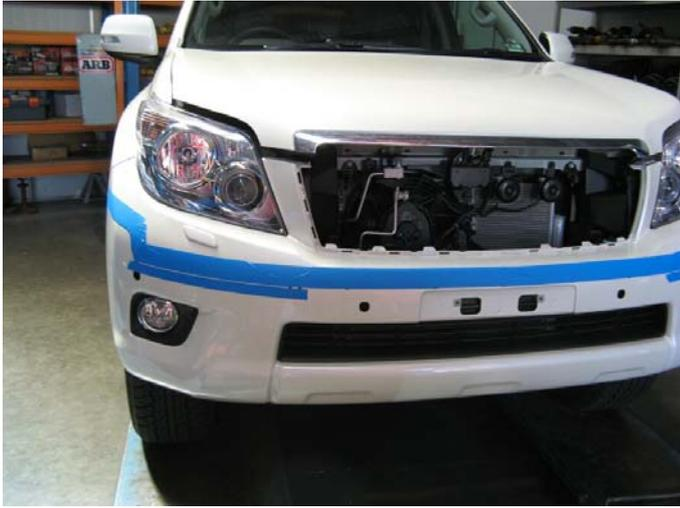
11. Note that the cutting line is co incident with the lower edge of the 50mm tape, ***this is critical.***
