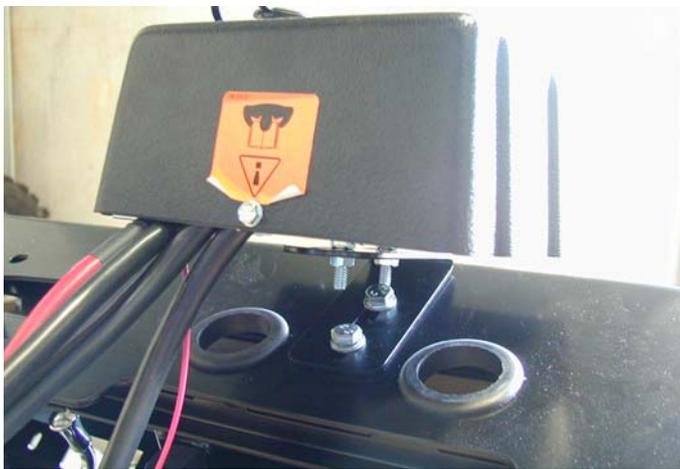
59. Attach the control box to the control box bracket as shown.
