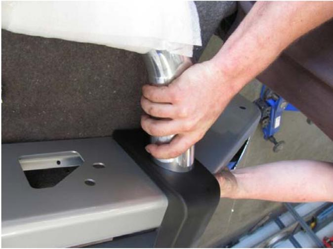
49. If fitting frame **P# 5121010**, locate frame as shown and then from below inside wings, secure with M12 x 50 bolts and washer sets
