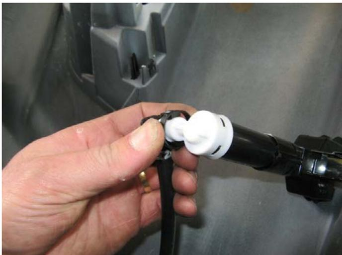
74. If headlamp washers are fitted, reconnect plumbing connections then attach the plumbing back to vehicle, routing rubber tubing along underside of vehicle grille crossmember, cable tie in position, **taking care not to apply too much squeeze on tube with cable ties, as this will cut off flow.**
