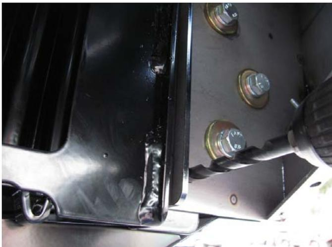
69. Using an electric drill and a Dia10.0 mm drill bit, drill two pinning bolt holes through the bull bar upright each side using the holes in the mount bracket flanges as a guide. One hole is located in the lower lug of the mount face and one up above the welded nuts. Use access through the light surround opening for the top hole.
