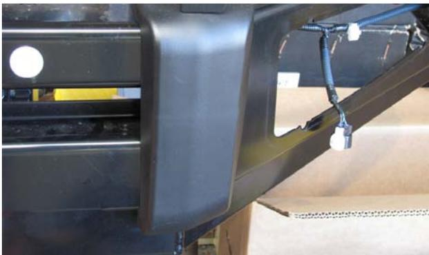
47. If fitting frame fit buffers with hole **5100020** to bar and secure using 6 x M6 flange nuts. If not fitting frame fit blank buffers **5100030**. Do not over tighten.
