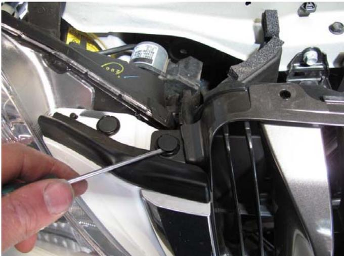
14. Remove the plastic scrivets securing the top of the grille
