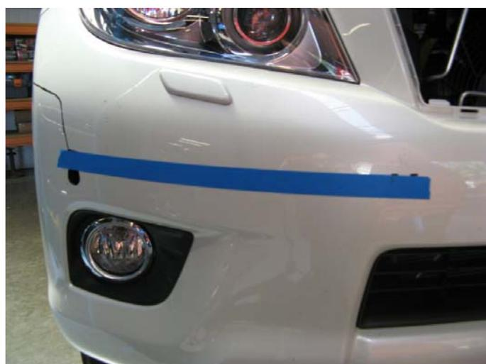
9. Apply some 25mm masking tape joining the cutting line positions from the most inboard position of the profile from the template to the mark on the outside of the 80mm marks across the centre of the bumper. Mark this line joining the two profiles, repeat for the other side of the bumper.
