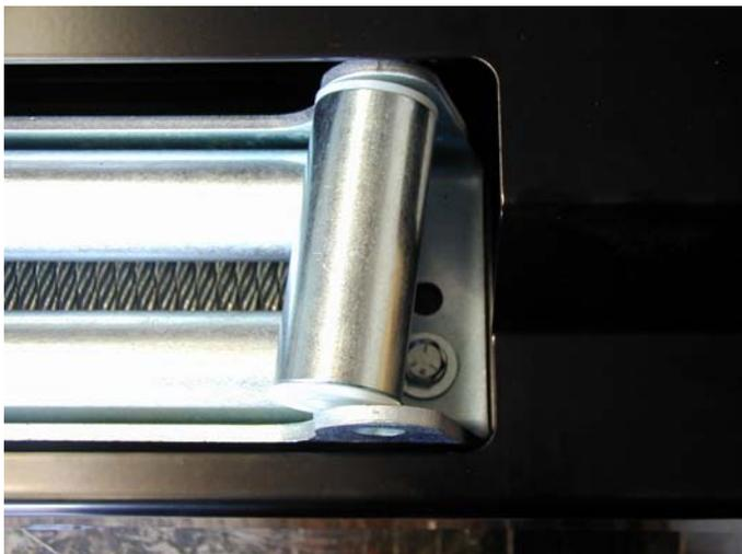
56. Remove the cir clips from the bottom of the vertical rollers of the fairlead and push the pin upwards. Push the vertical rollers inwards on the lower edges as shown and using two 3/8" x 1 3/4" bolts M10 flat and spring washers, attach the lower section of the roller fairlead to the bull bar and winch.
