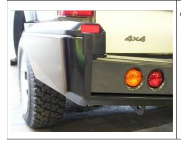
63. Fit reflector to buffer. Fit top edge in first and pivot downwards. Press in firmly.
