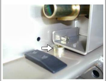
44. Place 8mm gold spacer between underside of centre cover panel and rear bar.
