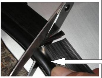
68. To fit rubber sealing strip to underside of front and rear of aluminium step plate, lay strips on the underside of step plate and place so over hang is even on both ends. Using scissors, cut darts up to the bulb end of the rubber strip, so the strips can follow the front and rear profile of the aluminium step plate.
