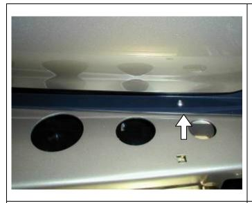
67. Using **M6 button head cap screws & M6 flange nuts,** fit top infill plate.
