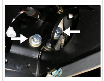
32. Use two **M14 x 40 bolt**, spring washer and large gold flat washer to secure rear bar side plate to side of chassis. (RHS shown)
