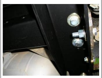
28. Fit three **M12 x 50 x 1.75 bolts**, spring washers and large gold flat washers to underside of chassis bracket.
