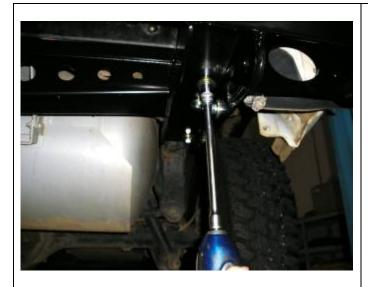
33. Tighten only M12 bolts from underside of chassis.
