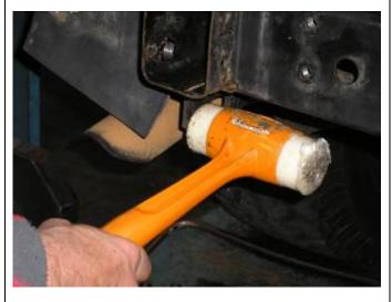
22. Hammer out tie down plates to allow for bar fitment.
