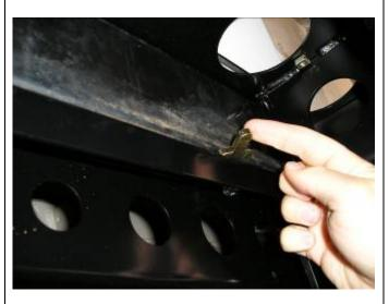
30. Insert spacer between rear bar and vehicle crossmember as shown. Align hole with nut plate previously inserted in crossmember.
