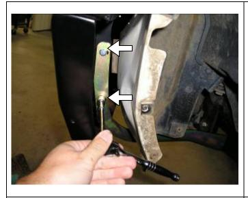
52. Using **M8 x 25 bolts**, flat washers and flange nuts secure end surrounds to braces finger tight. (RHS shown.)
