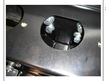
27. Use four M12 x 35 x 1.25 bolts, spring washers and flat washers to fit rear bar to rear crossmember. Secure finger tight only. If fitting a swing away wheel carrier to vehicle, use the two remaining 12mm x 35 mm x 1.25 bolts etc to bolt the locator bracket to front of rear bar.
