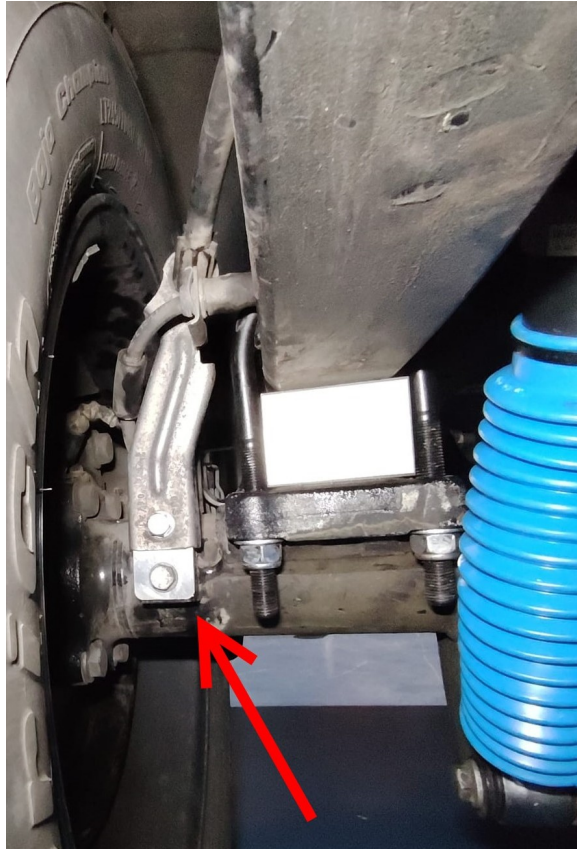
Fig. 3: correct installation of rear brakeline relocation brackets
